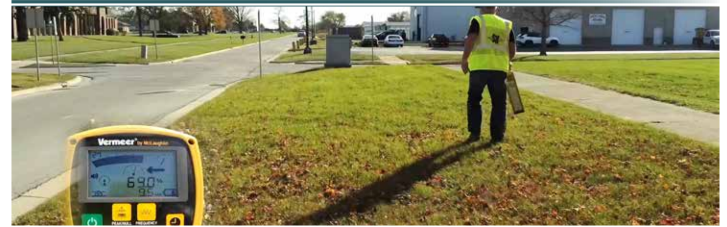
Figure 62: The line once again shifts directions and veers gradually back to the west side of the main. Notice the angle of the compass.
