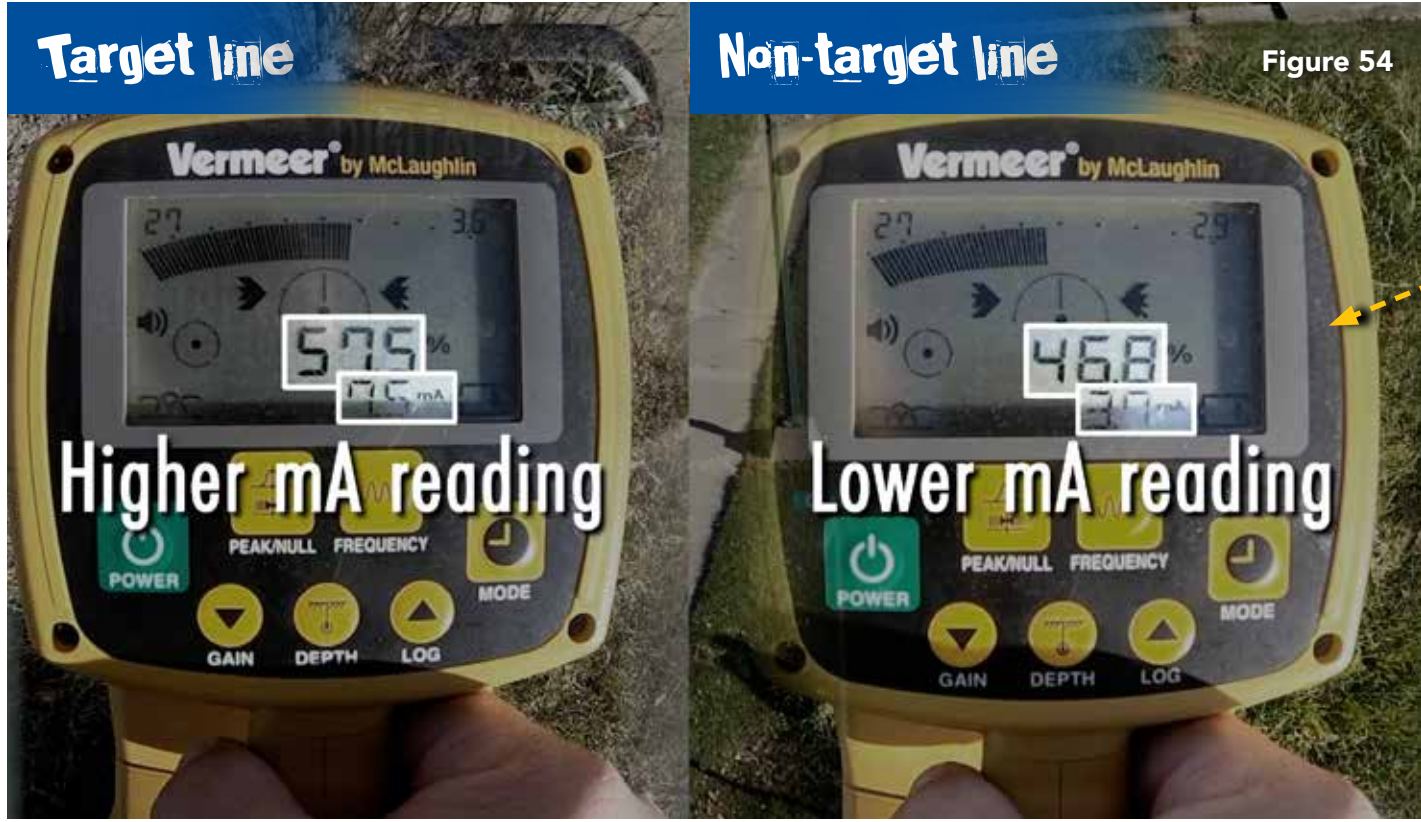
In Figure 53 , the receiver is held over two different buried lines. The gain is set at a level of 27 over both lines. The photo on left indicates a signal strength of 57.5 over a line 3.6' deep. The photo on the right shows a signal strength of 46.8 over a line 2.9' deep.
