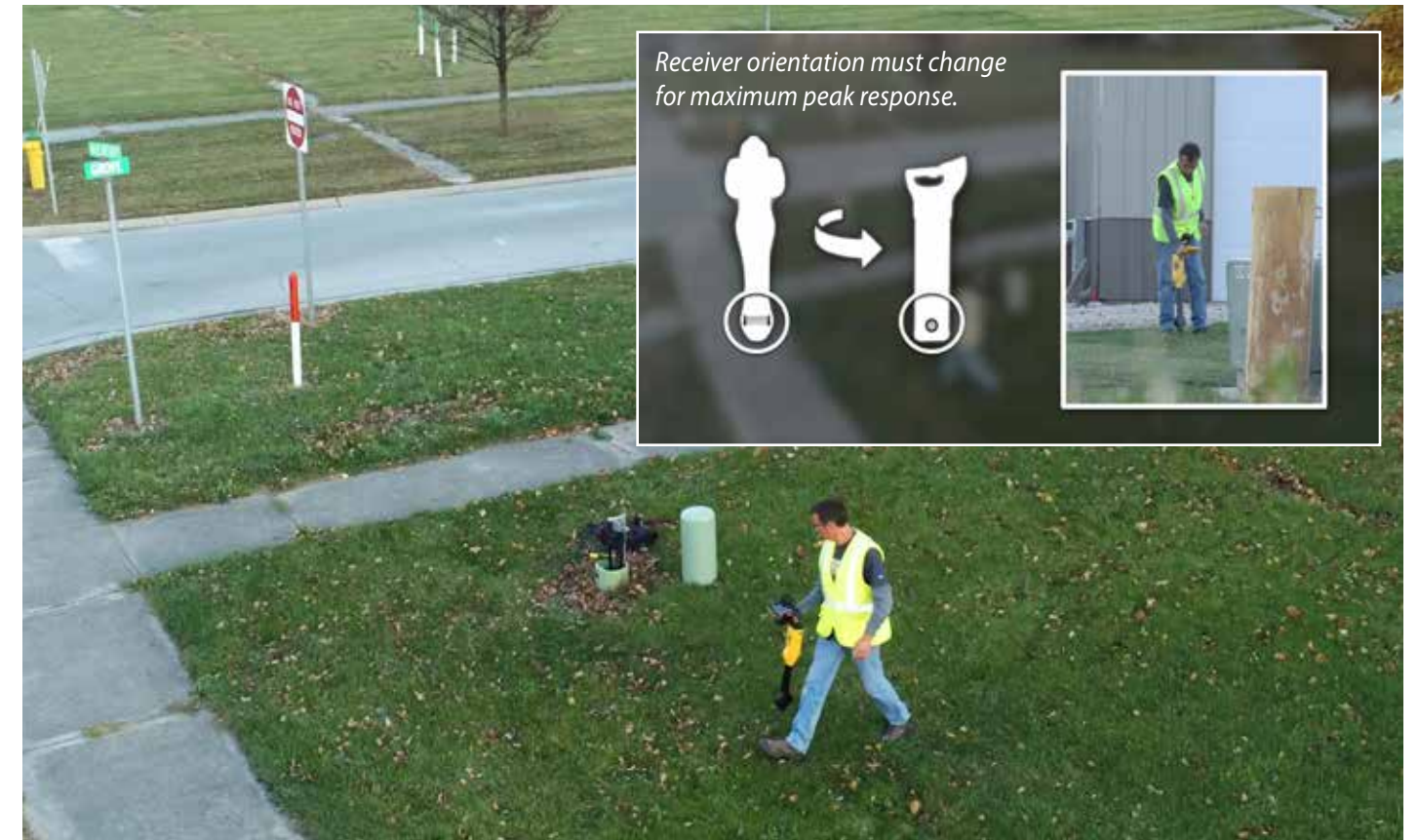
Figure 44: 270 degrees around the access point. The sweep is complete once back to the starting point.
