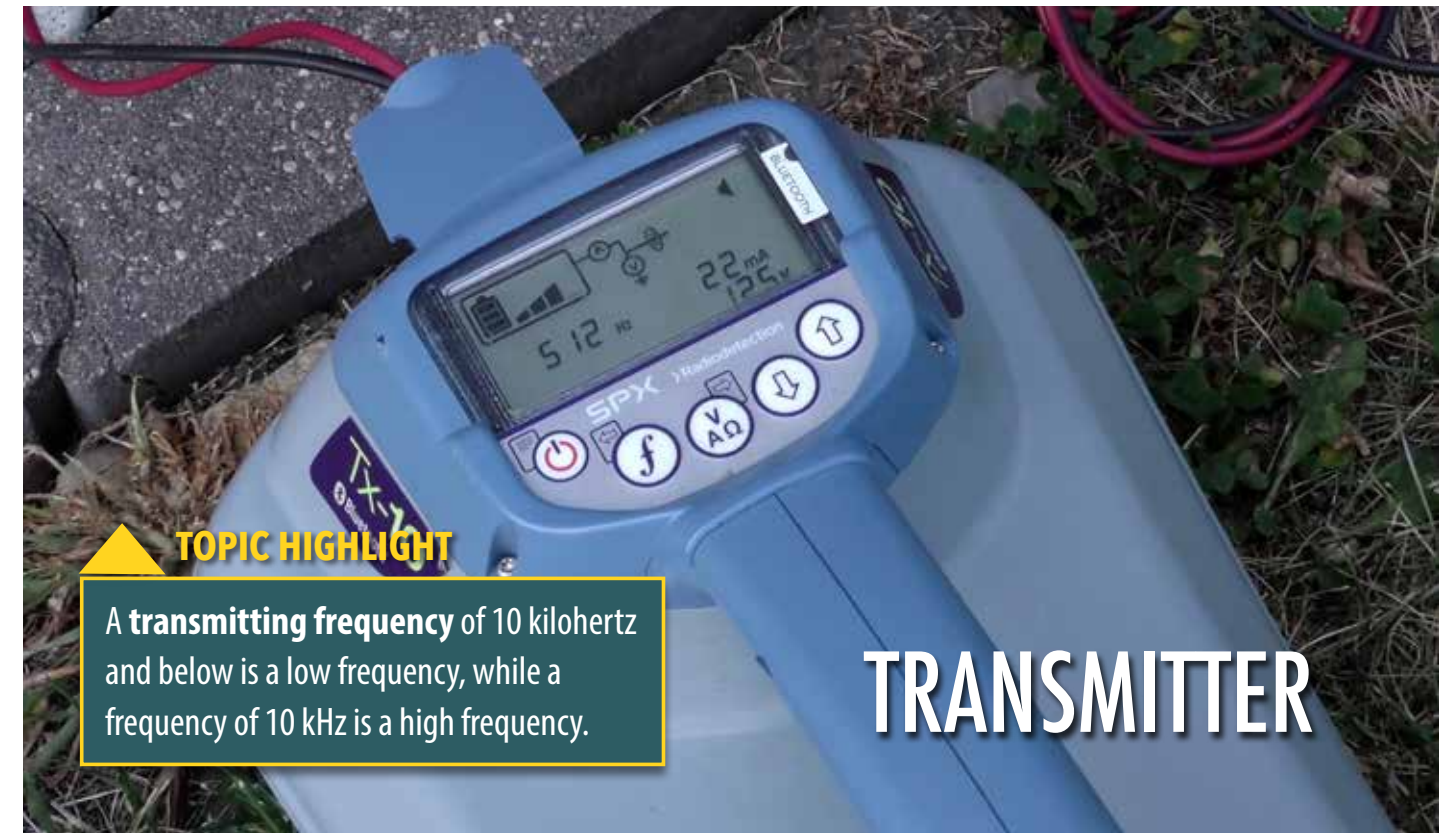
Figure 2: Current is produced by the transmitter. As current flows on a conductor, an electromagnetic field is produced.
