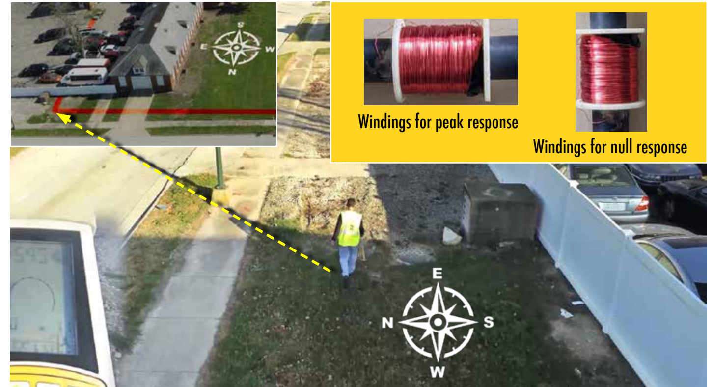
Figure 58: Excessive swinging of the receiver creates the possibility of missing turns in the target line and instead continuing forward on a non-target line.
