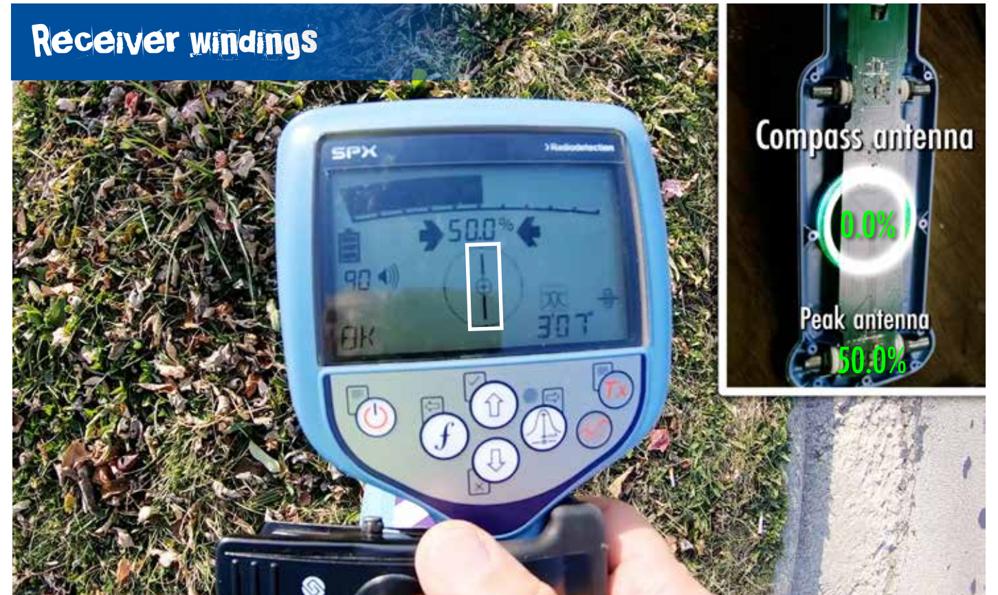
Figure 54: When the compass antenna receives no signal, the indicator on the display is in line with the line being located.
