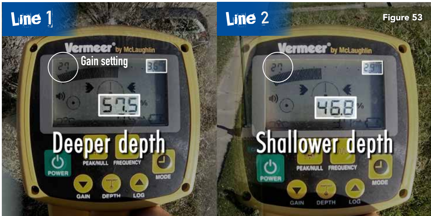
In Figure 53 , the receiver is held over two different buried lines. The gain is set at a level of 27 over both lines. The photo on left indicates a signal strength of 57.5 over a line 3.6' deep. The photo on the right shows a signal strength of 46.8 over a line 2.9' deep.
