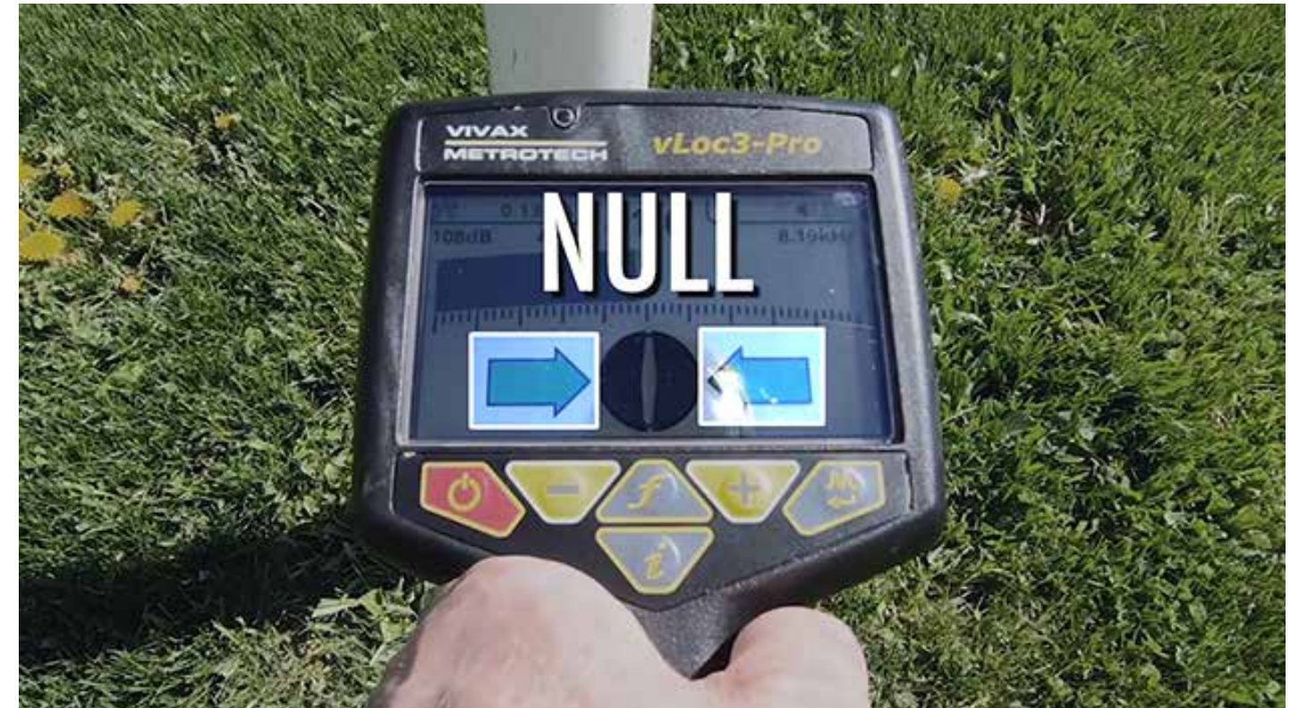
Figure 14: Null is typically shown with arrow icons. One visible arrow represents an imbalance that indicates the direction the operator should move the receiver toward. Two visible and opposite arrows represents that a null balance has been achieved.
