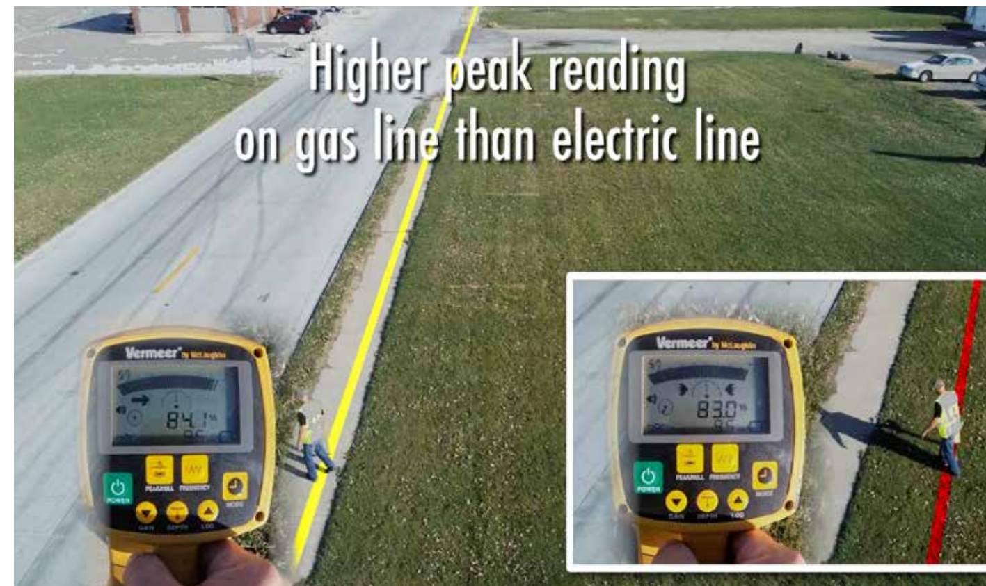
Figure 72: We have a peak and null over the electric and a high peak reading without a null over the gas.
