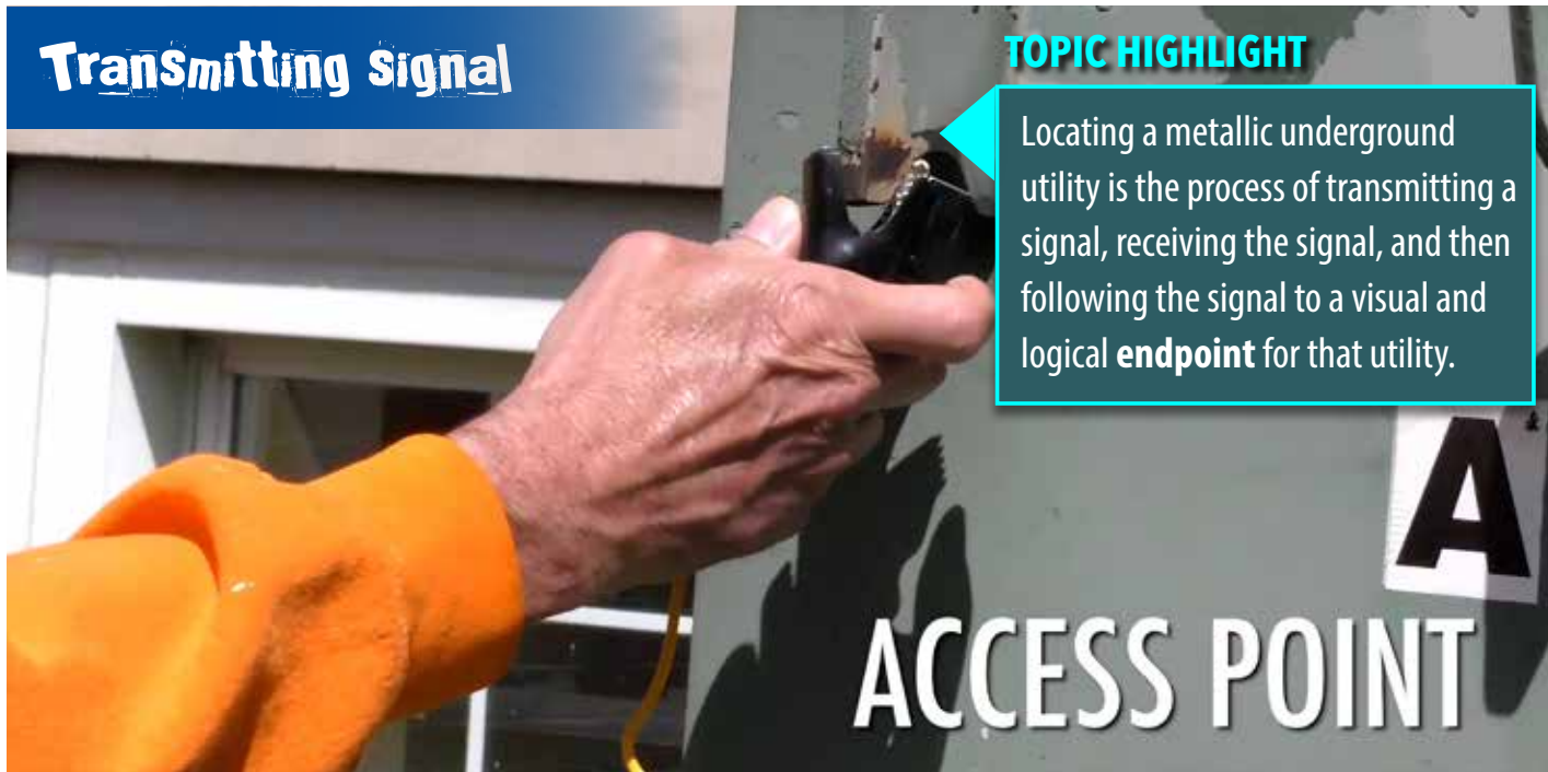
Figure 4: Attaching a cable from the transmitter to an electric transformer.
