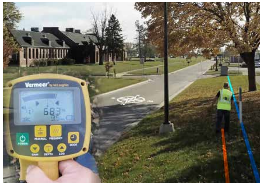
Figure 61: Locating east of the water main. The compass indicator on the receiver can show a change in direction of the target line.
