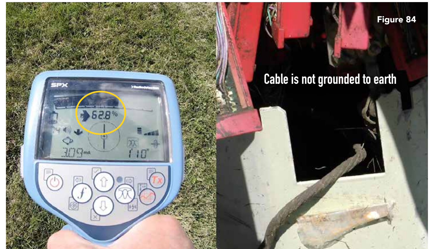
Watch our signal strength at the far-end as we take the ground off of this cable, so that it will no longer send signal to earth ( Figure 83 ). There is a significant drop in signal strength ( Figure 84 ), because now the far-end is not grounded.
