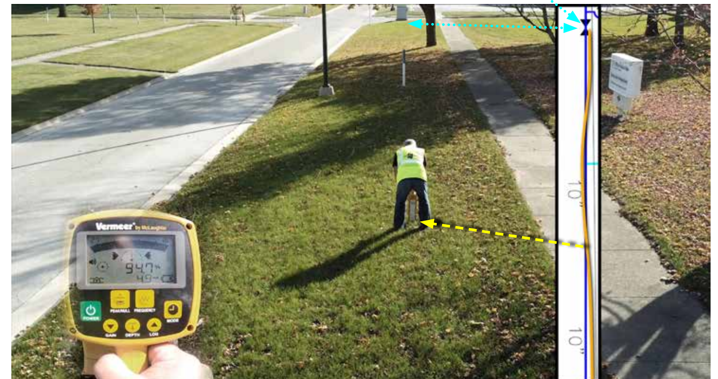
Figure 64: The overall path of the water line (blue) and target cable line (orange) can be seen on the map to the right.
