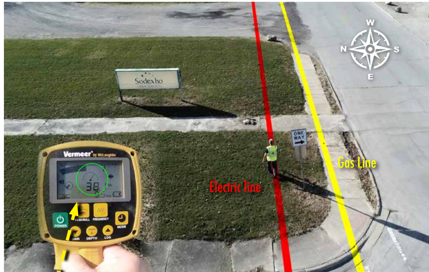
Figure 67: The receiver in this image shows a change in direction, complicating the locate.
