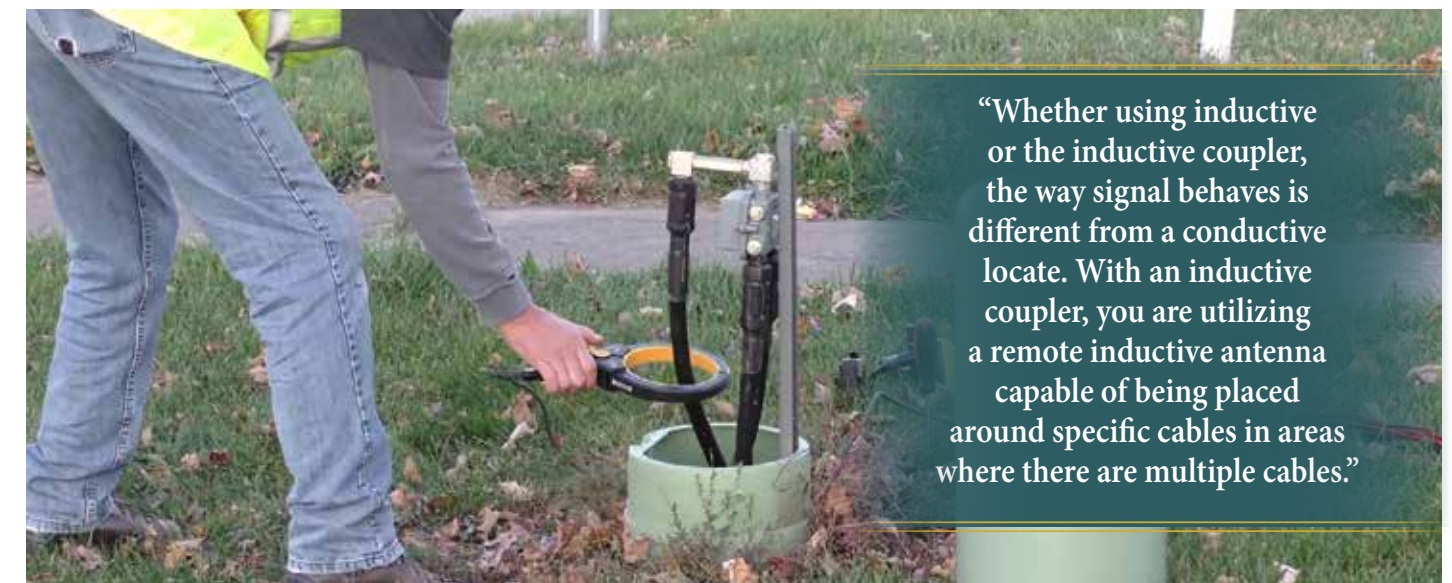
Figure 10: An inductive coupler being used to locate a cable TV feeder.
