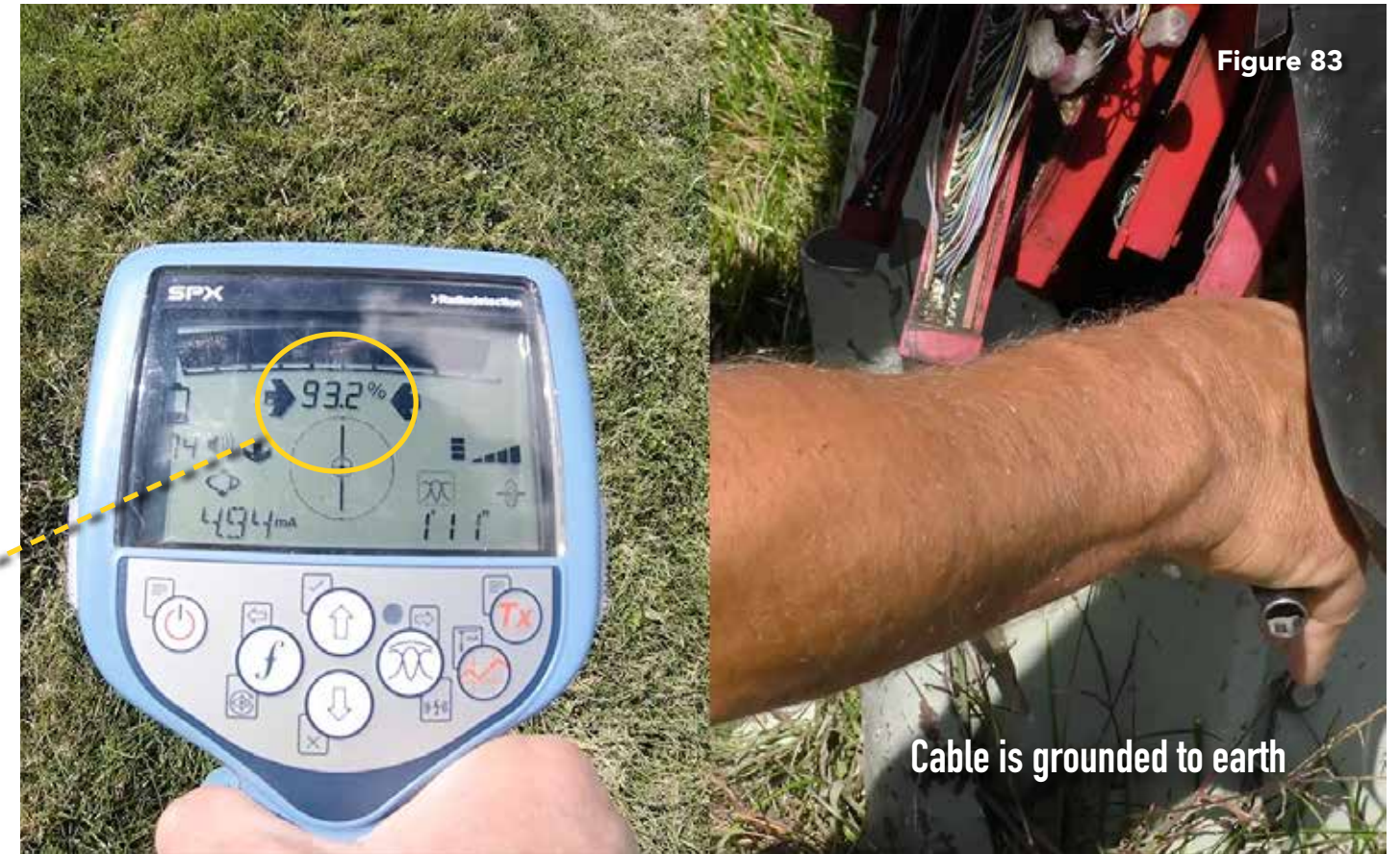
Watch our signal strength at the far-end as we take the ground off of this cable, so that it will no longer send signal to earth ( Figure 83 ). There is a significant drop in signal strength ( Figure 84 ), because now the far-end is not grounded.
