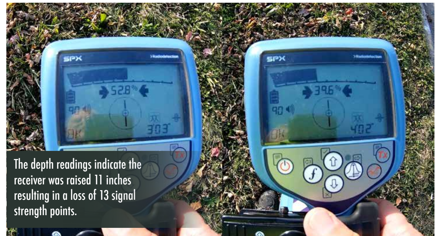
Figure 15: On the left, the strength of the field at ground level is stronger than on the right where the receiver is held higher.
