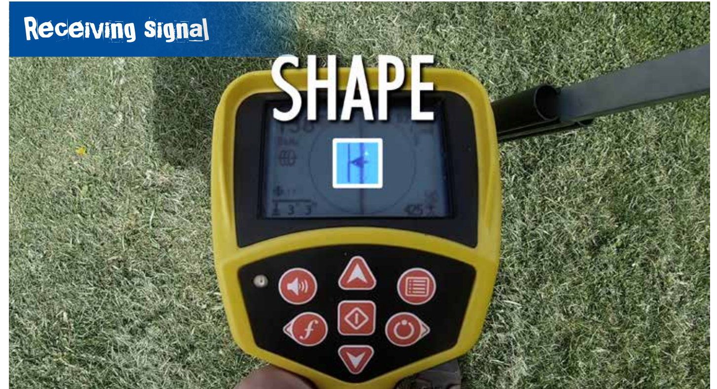
Figure 6: Arrows provide left-right guidance and this guidance is known as a null reading. Peak and null readings are compared to each other to determine the shape of the electromagnetic field being received.
