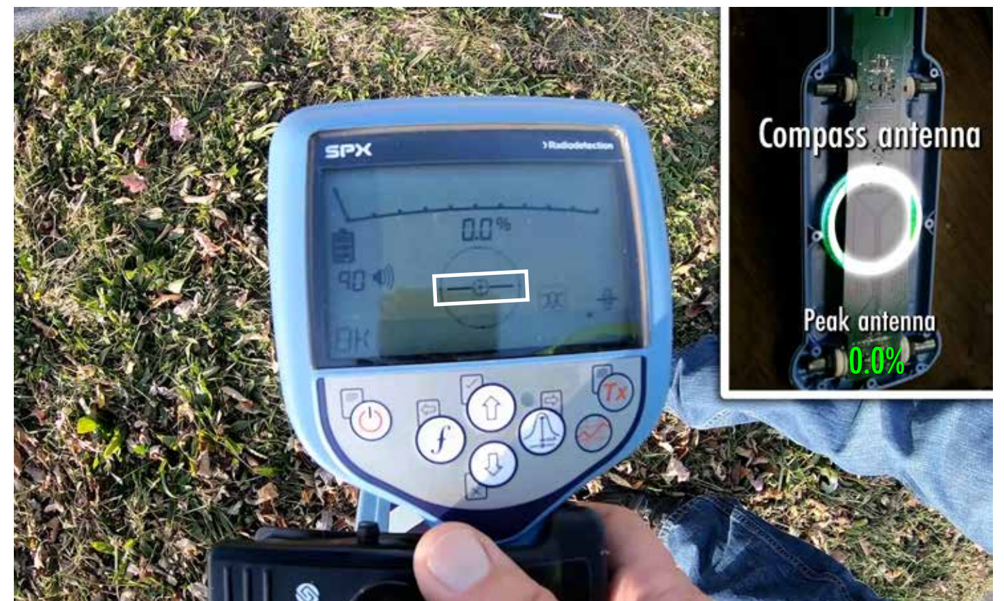
Figure 55: When the compass antenna receives maximum signal, the indicator is horizontal on the display.
