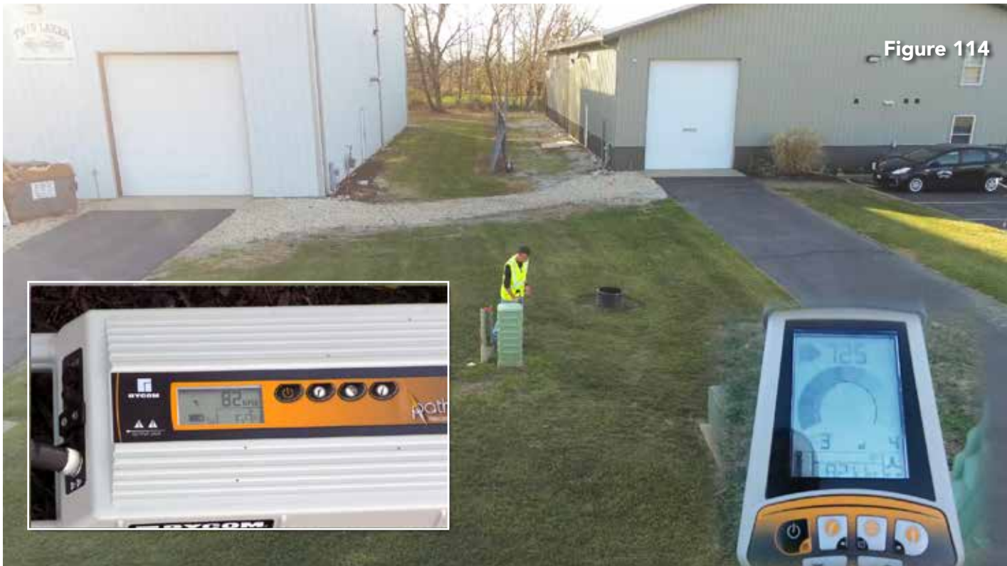
Using the transmitter frequency 82 kHz, the connection to the unused pairs leads directly the logical and visual endpoint—the telephone pedestal (Figure 114). With the receiver beyond the pedestal and over the electric line, there is no null response (Figure 115). A “peak but no null response” is the result of a very low amount of signal on the electric line.
