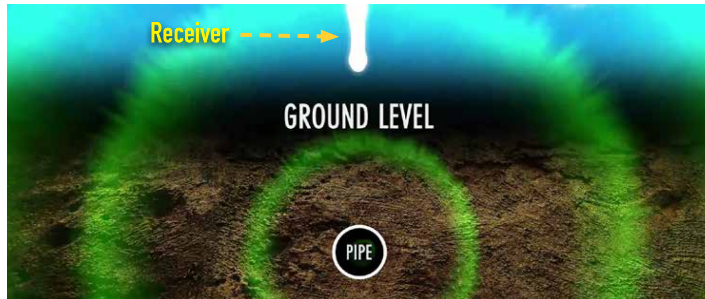
Figure 11: Signal circles are created by flowing alternating current on the metallic skin of a pipe or cable.
