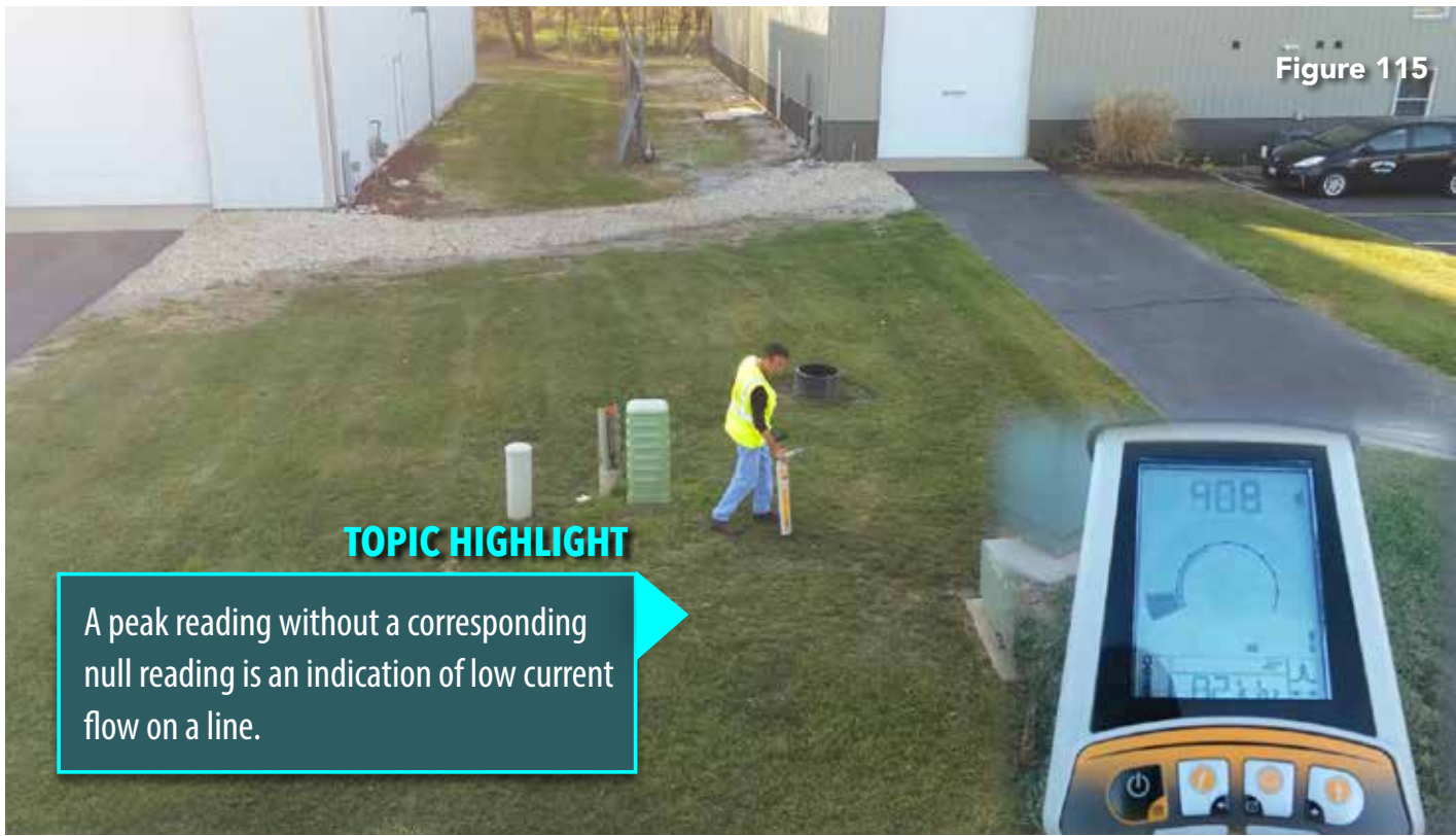
Using the transmitter frequency 82 kHz, the connection to the unused pairs leads directly the logical and visual endpoint—the telephone pedestal (Figure 114). With the receiver beyond the pedestal and over the electric line, there is no null response (Figure 115). A “peak but no null response” is the result of a very low amount of signal on the electric line.
