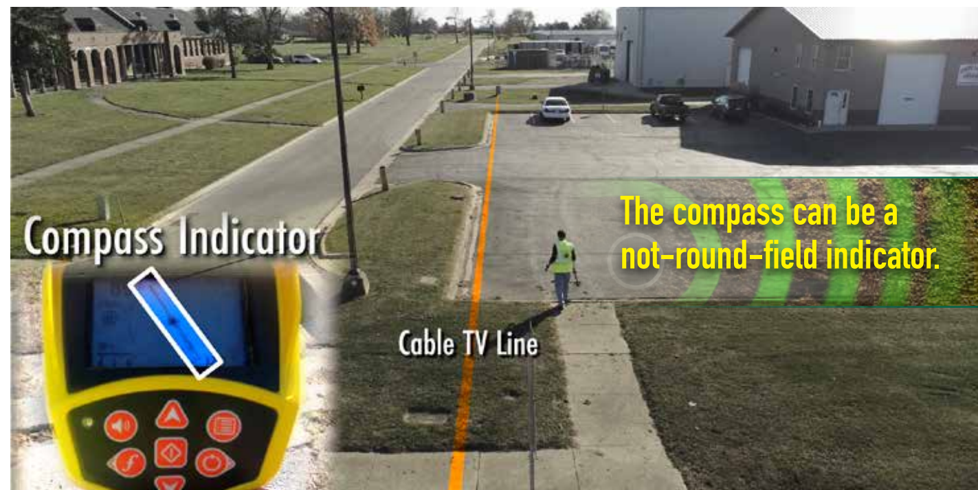
Figure 66: The energized cable TV line running parallel and to the east of the water main heavily influences the compass indicator while the water main is being located.
