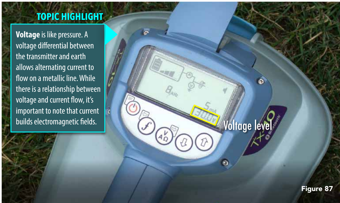
We're locating an insulated tracer wire on 8 kHz at the second level of power. We only have 5mA of current flow leaving the transmitter (Figure 86). We're going to turn up the transmitter to the third level of power, and we still only have 5 mA (Figure 87).
