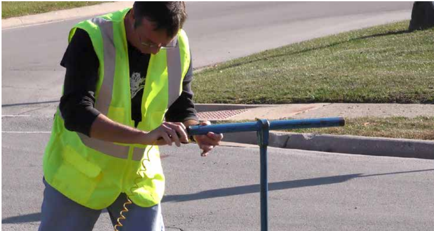
Figure 20: A conductive connection to a wrench that is seated on a water main valve.
